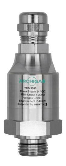
The compact and robust TCD3000 SiA (Screw-in) is ideally suited for precise, fast, and sensitive measurement of (quasi-)binary gas mixtures. The measurement is based on the principle of thermal conductivity. This technology is ideal for measuring gases with significantly different thermal conductivities, such as  $H_2$  and  $O_2$ .
